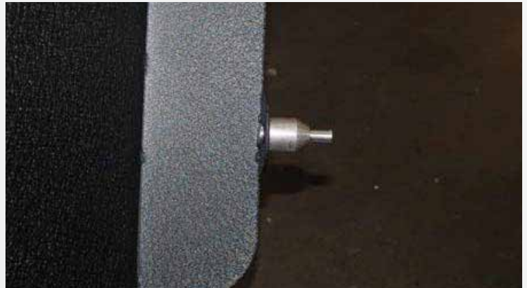
Use the supplied Phillips screw and install the supplied aluminum pin into the bottom of the black metal air filter shield, pointing down
