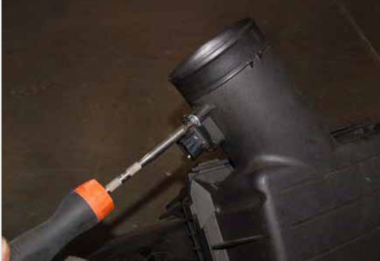
Using a Torx T20 bit, remove the Mass Air Sensor.
