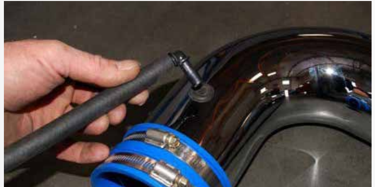
Install the supplied grommet in the bottom of the chrome inlet tube for the breather hose. Install the black plastic 90 degree fitting into the supplied 3/8" hose and push other end of Fitting into grommet. Install blue connector and clamps onto throttle body side of the tube.
